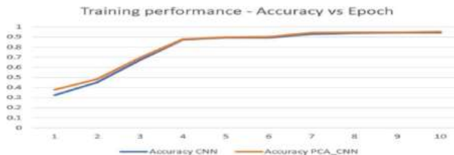
Fig. 5. Training accuracy of the plain CNN versus the CNN with PCA over ten epochs.
