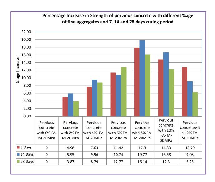
Figure 2: Variation of Increase in in Strength of pervious concrete with different %age of fine aggregates and 7, 14 and 28 days curing period
