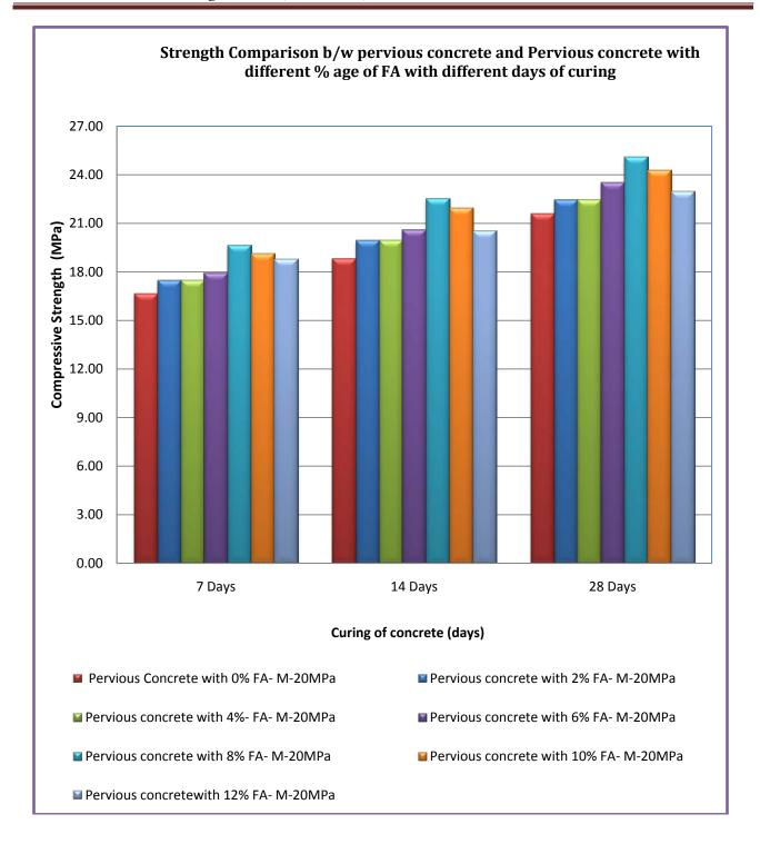
Figure 1: Strength of pervious concrete with different %age of fine aggregate.
