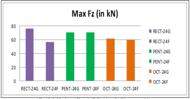
Graph 6: Maximum Shear in Z directions for 24storey models.
