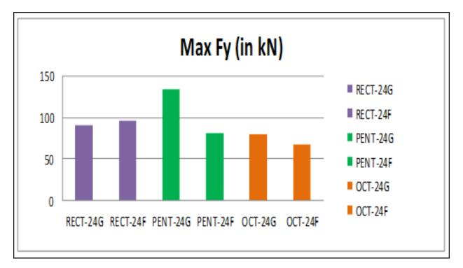
Graph 5: Maximum Shear in Y directions for 24storey models.
