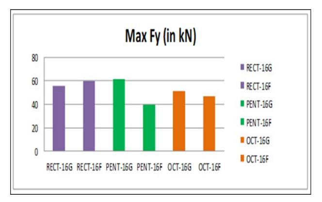
Graph 2: Maximum Shear in Y directions for 16storey models.
