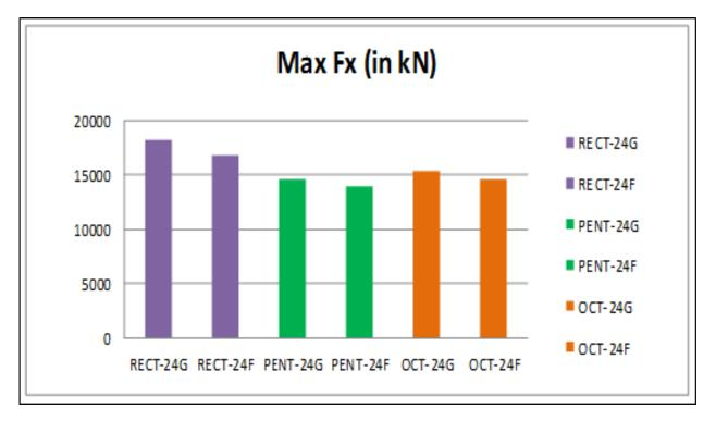
Graph 4: Maximum Shear in X directions for 24storey models.
