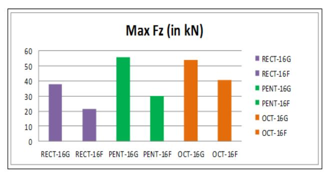
Graph 3: Maximum Shear in Z directions for 16storey models.
