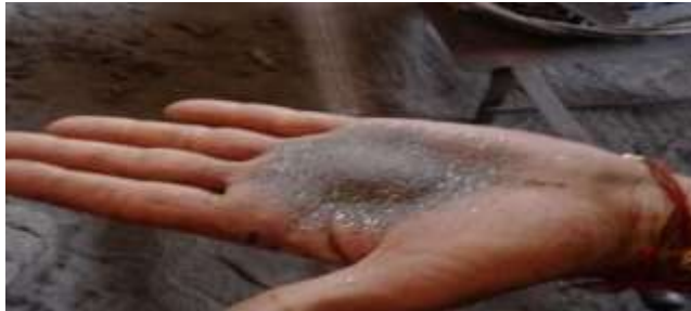
Figure 3: Foundry Sand Sample.
