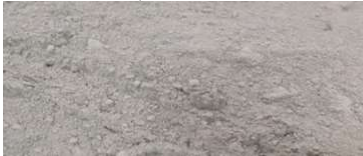
Figure 2: Grade 53 Ordinary Portland cement Sample.
